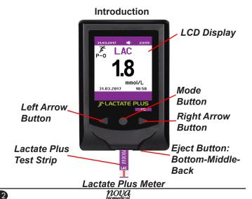
The Lactate Plus Meter is a hand-held testing device that measures lactate (LAC) in whole blood. The test strip is touched to a drop of blood to initiate the test process.
